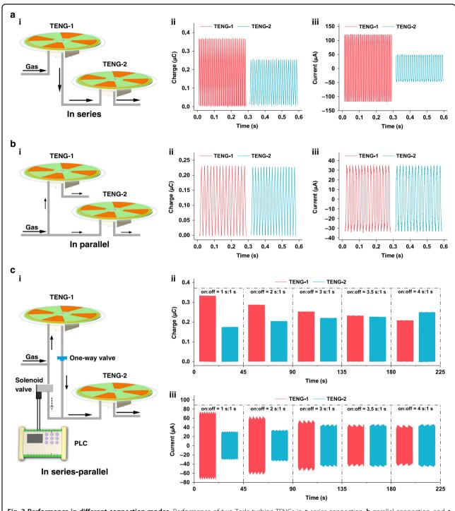
**Fig. 3 Performance in different connection modes.** Performance of two Tesla turbine TENGs in **a** series connection, **b** parallel connection, and **c** series-parallel connection modes. (i) Schematic diagram. (ii) Transferred charge. (iii) Short-circuit current.
