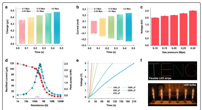
Fig. 2 Basic performance of the Tesla turbine TENG. a Transferred charge. b Short-circuit current. c Open-circuit voltage. d Rectified current and peak power with different external resistances at gas pressures of 0.12–0.13 MPa. e Charging performance with different capacitors at gas pressures of 0.12–0.13 MPa. f Video captures of lighting the flexible LED strips and the LED bulbs at gas pressures of ~0.18–0.2 MPa.
