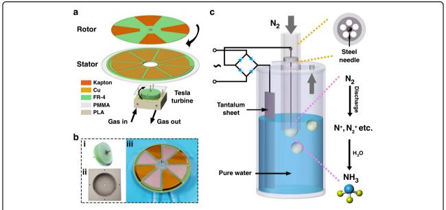
Fig. 1 Schematic diagrams and photographs. a Schematic diagram of the Tesla turbine TENG. b Photographs of (i) the bladeless turbine with the driving shaft, (ii) the 3D printing casing, and (iii) the disk TENG. c Schematic diagram of the ammonia synthesis device and main reaction processes.
