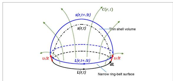
Figure A1. Schematic diagram showing the movement of a volume and its surface from time t to time  $t + \Delta t$ , where the thin shell volume unit and the belt-like surface area unit will be used for the mathematical derivation.
