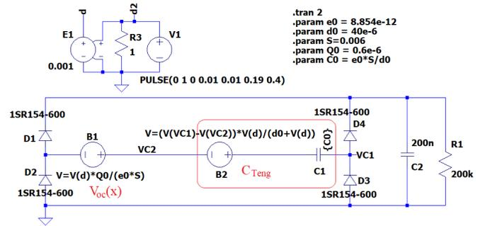
Fig. 4: LTspice model for a TENG with a full bridge rectifier
