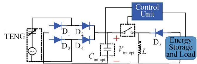
Fig. 14: A PMS based on a buck-boost converter [99]
