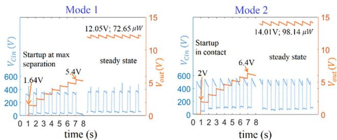
Fig. 18. Two modes of startup and steady state responses [54]
