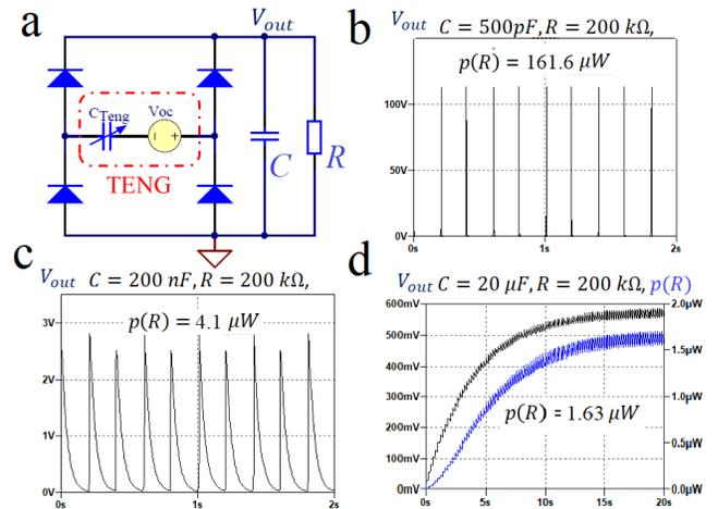
Fig. 5. (a) Circuit model of TENG with a full wave rectifier and a capacitive filter. (b)- (d): Output voltage and power under 3 values of filter capacitance: 500 pF (b), 200 nF (c), 20  $\mu\text{F}$  (d).
