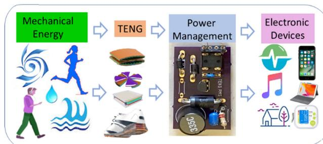
Fig. 1. Illustration of a self-powered system using energy harvested with TENGs. A power management system is needed to convert the TENG's output into a regulated form suitable for electronic devices.
