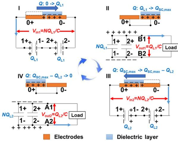
Fig. 10. Switched capacitors for a sliding mode TENG [95]
