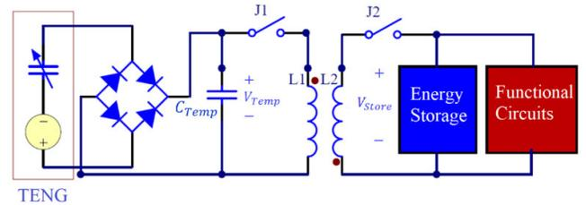
Fig. 12. A PMS based on a flyback converter [72]
