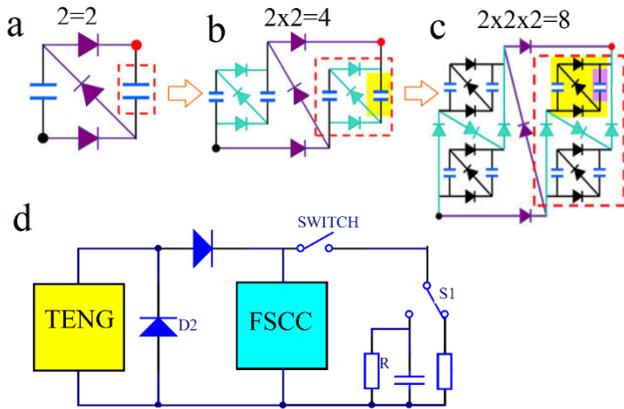
Fig. 11. (a),(b),(c), Fractal design of switching capacitors. (d): a PMS based on fractal switching capacitors [96]
