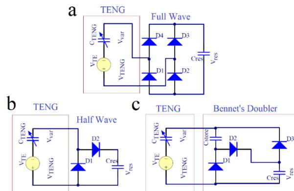
Fig. 7. Three rectifying topologies for storing energy in a capacitor
