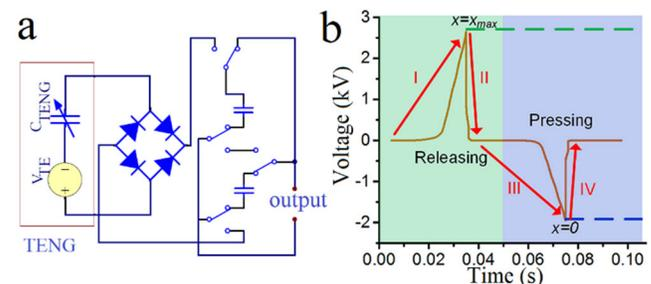
Fig. 9. (a) Stepping down the voltage with switched capacitors [94], (b) Four phases of a motion cycle [85]
