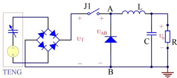
Fig. 13. A PMS based on a buck converter
