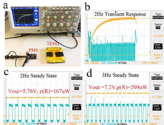
Fig. 17. (a) TENG and PMS prototype in an experiment setup; (b)-(d) Output voltage  $V_{out}$  (orange) and  $V_{Cin}$ (green) at 2Hz and 3Hz TENG frequency
