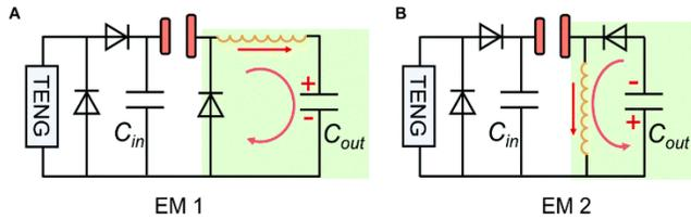
Fig. 20. PMS in [101] based on a buck converter (A) and a flyback converter (B) with spark switch
