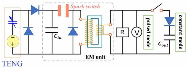
Fig. 19. A PMS with a spark switch [53]
