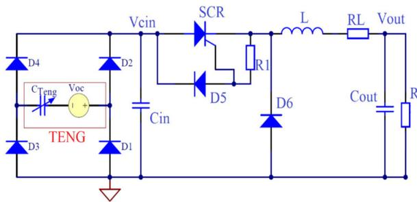
Fig. 16. Complete circuit of the PMS in [51]
