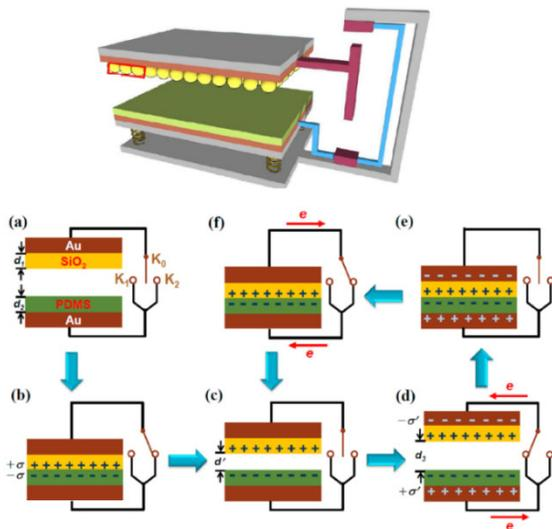
Fig. 6. A TENG with a mechanical switch, and the operation of the switch [52]
