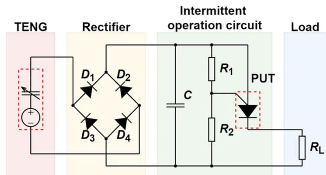
Fig. 15: A PMS with a passive switch using programmable unijunction transistor (PUT) [100]
